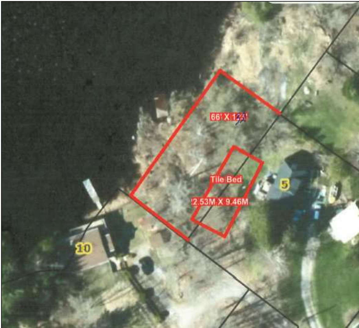
Figure 3: Existing Septic System
